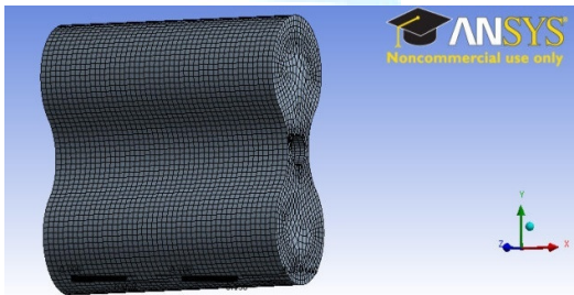
Fig .2 FE model meshing of lobe blower
